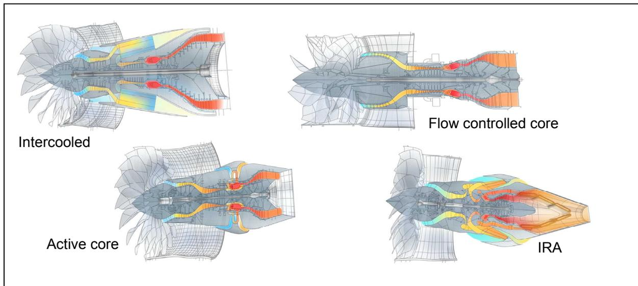
Figure 2 – The Four Original NEWAC Advanced Cycle Concepts
